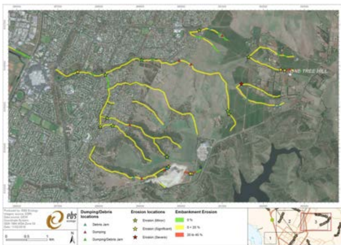
Figure 5.29 Erosion locations (eastern portion of catchment)
