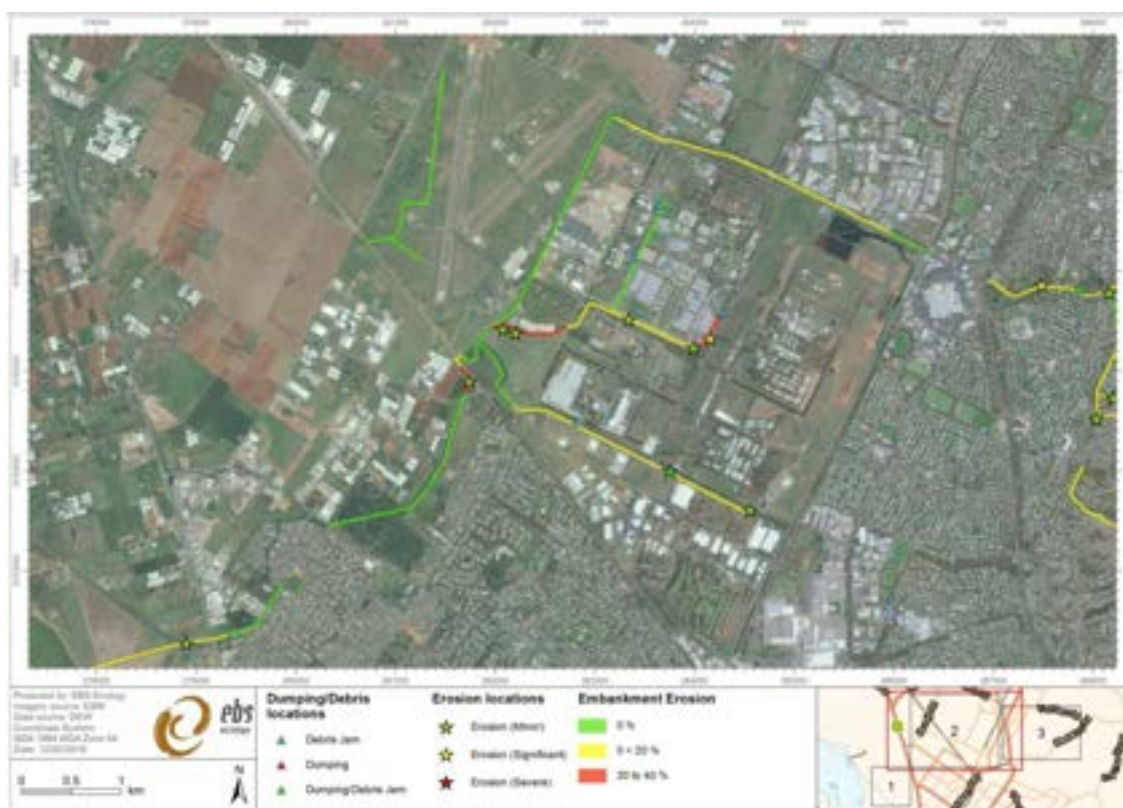
Figure 5.30 Erosion locations (central portion of catchment)
