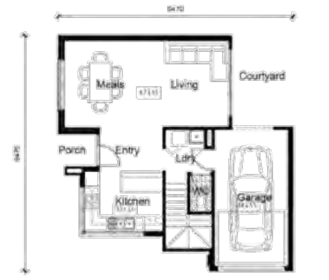
GROUND FLOOR PLAN DWELLING TYPE 1 Ground Floor 36.40m 2 First Floor 62.51m 2 Garage 12.45m 2 Bakery 6.06m 2 Porch 1.71m 2 Total 122.53m 2
