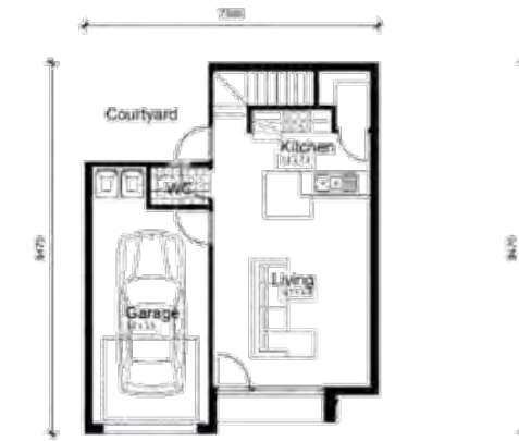
GROUND FLOOR PLAN DWELLING TYPE 2 Ground Floor 38.70m 2 First Floor 48.61m 2 Garage 20.31m 2 Bakery 9.80m 2 Porch 2.94m 2 Total 117.96m 2
