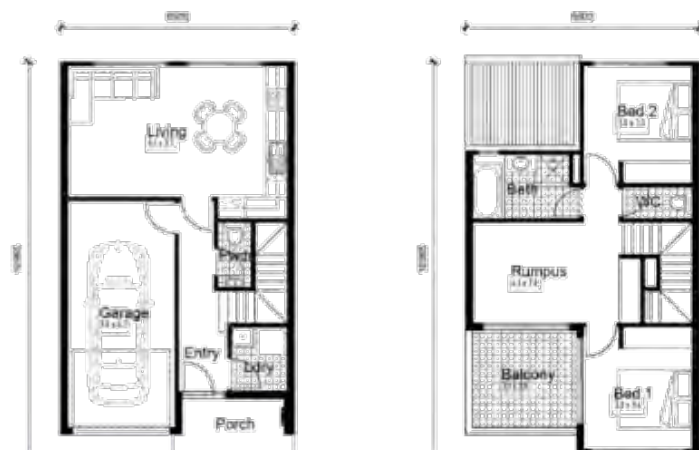
GROUND FLOOR PLAN DWELLING TYPE 6 Ground Floor 43.34m 2 First Floor 52.59m 2 Garage 20.50m 2
