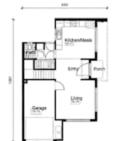
GROUND FLOOR PLAN DWELLING TYPE 7 Ground Floor 52.18m 2 First Floor 46.47m 2 Garage 20.61m 2
