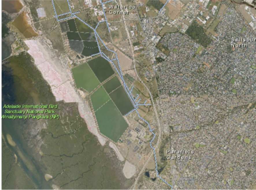
Figure 5: Extent of the Recycled Water Network (Source Location SA)
